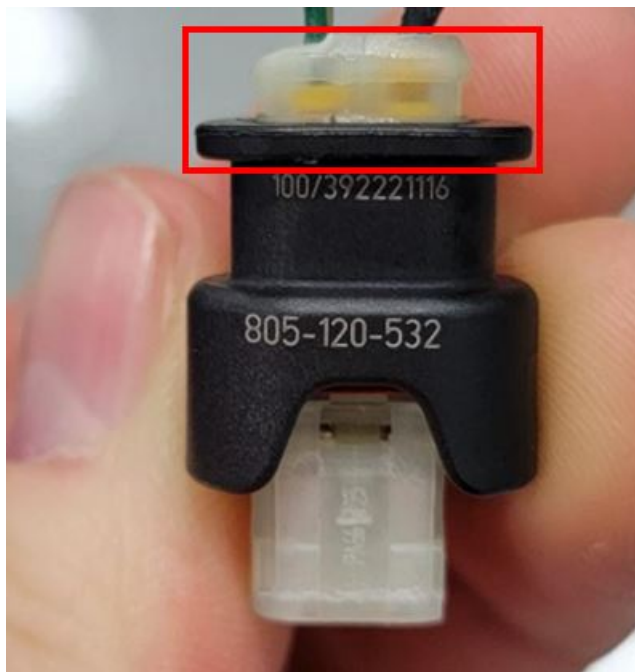
Fig. 3 Connector (D3157A) Not Fully Seated
