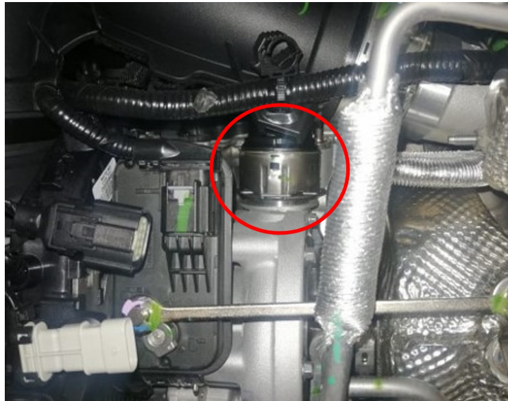
Fig. 3 Fully Secured And Locked Quick Connect
