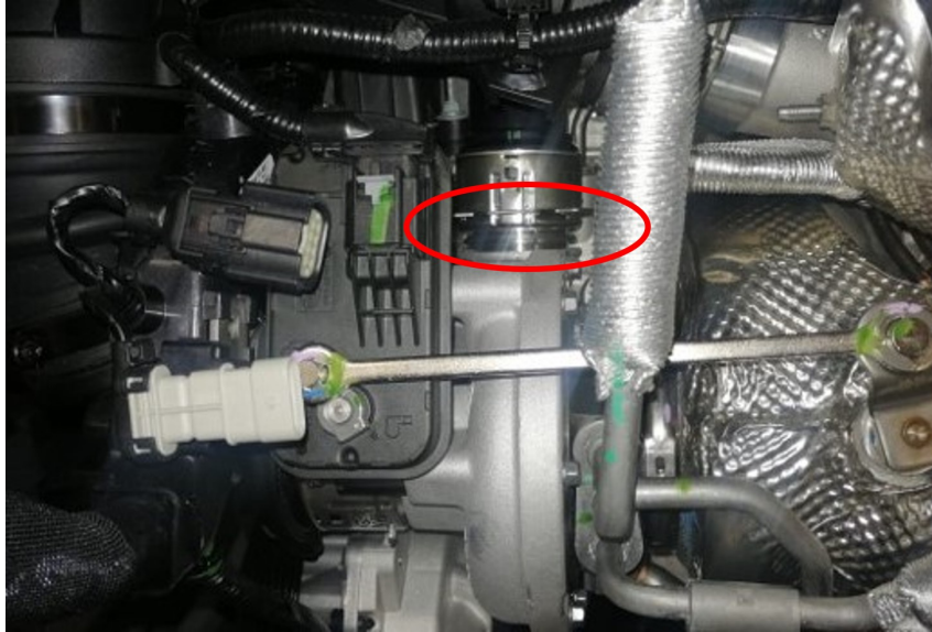
Fig. 5 Quick Connect Not Fully Seated
