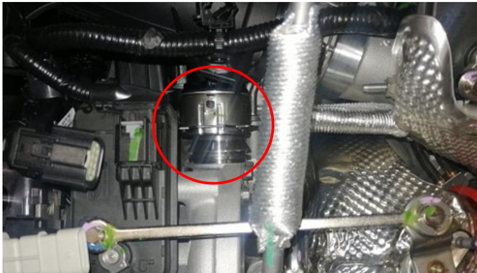
Fig. 4 Quick Connect Completely Disconnected
