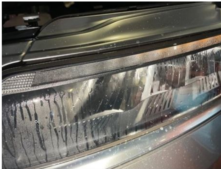
Fig. 1 Water In The Headlamp Assembly
