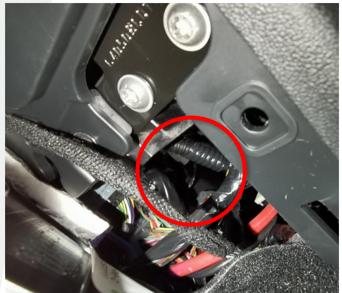
✗ Figure 4 – Knee impact foam is missing
