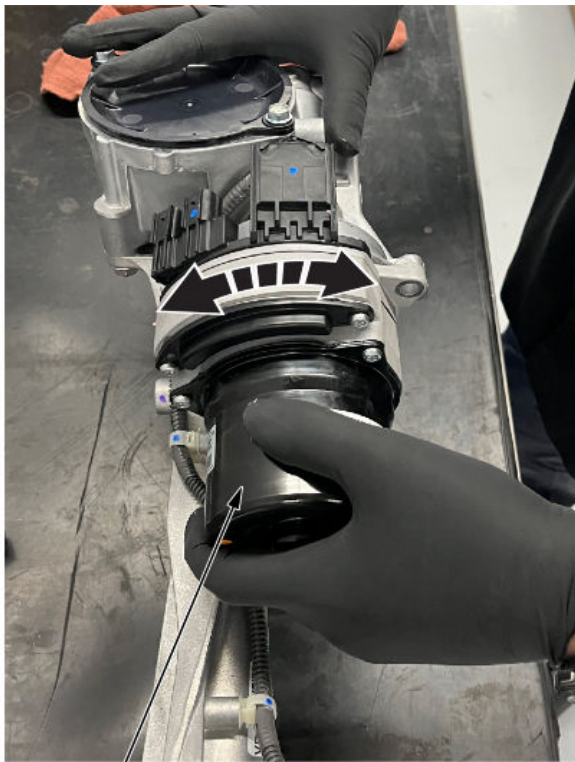
EPS MOTOR CONTROL UNIT Turn unit two or three times to the right and left (about 45 degrees).
