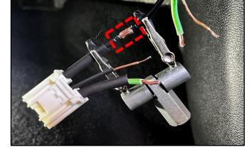
9. Heat the joint with a soldering iron from underneath the wires while applying solder to the top until molten solder melts into the jointed wires, as shown. Repeat for all three (3) wires.
