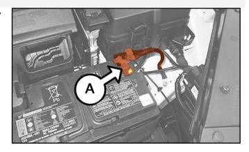
2. Detach/open the battery positive (+) terminal cover (B).
