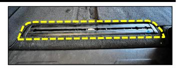
6. Insert the reinforcement plate into the seat rail as shown
