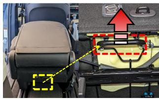
4a. Remove the four (4) left <u>outer</u> seat rail T50 retaining bolts.
