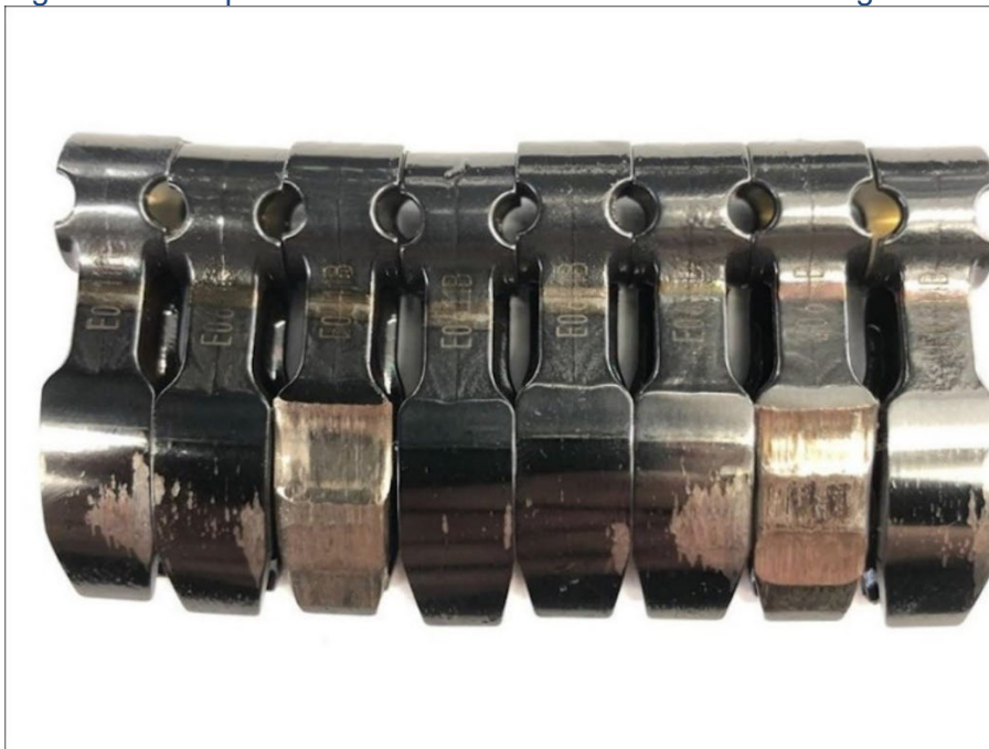
Figure 2: Examples of rocker arms with worn surface coating:
