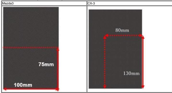
7. Cut the sheet into half (75mm X 100mm) for Mazda3 or 130 mm X 80mm for CX-3.
