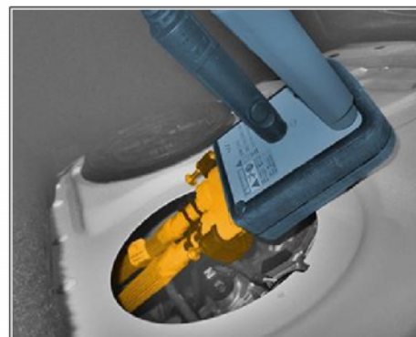
Rear power electronics traction line
