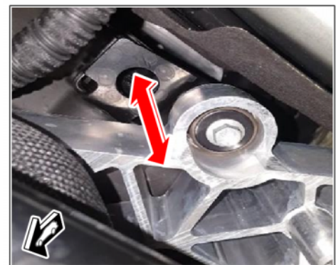
Inspection for tightness
