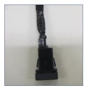
2. After reaching the border between the thick rubber foam and the harness, cut the tape once. Then, start wrapping again in the reverse direction (i.e. start from where the tape was cut and stop at the middle of the switch). After cutting the tape once more, wrap upwards again to ensure no gaps are left.
