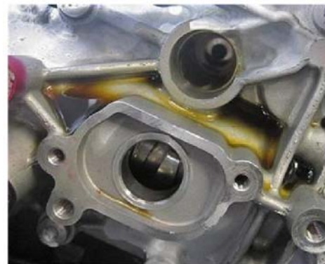
Fault type 2: Cylinder head cover leaking
