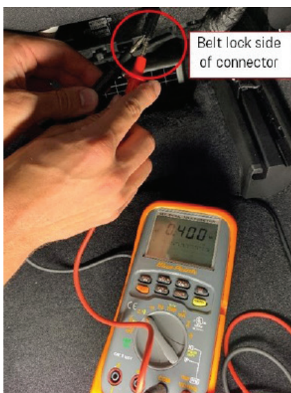
Figure 3: Resistance check for (4a)
