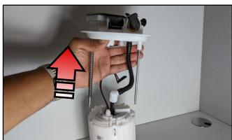
6c. Separate the upper fuel pump module plate from the lower body.
