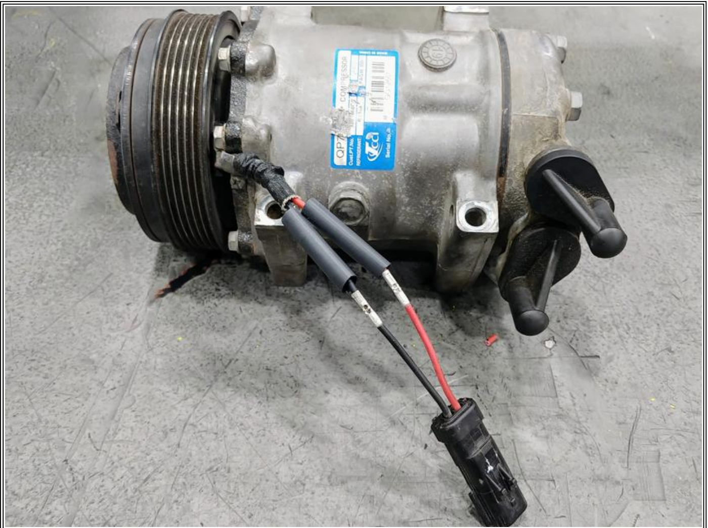
Figure 3: Pigtail from failed compressor spliced on to replacement compressor
