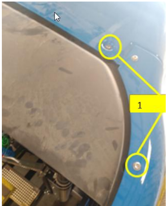
Figure 5: Air deflector extension topside bolt placement.
