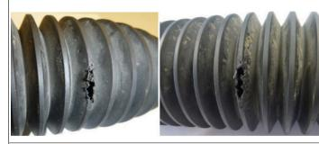
Corrosion / water ingress due to damaged boot (animal bite).
