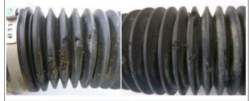
Corrosion / water ingress due to damaged boot (high pressure cleaner).
