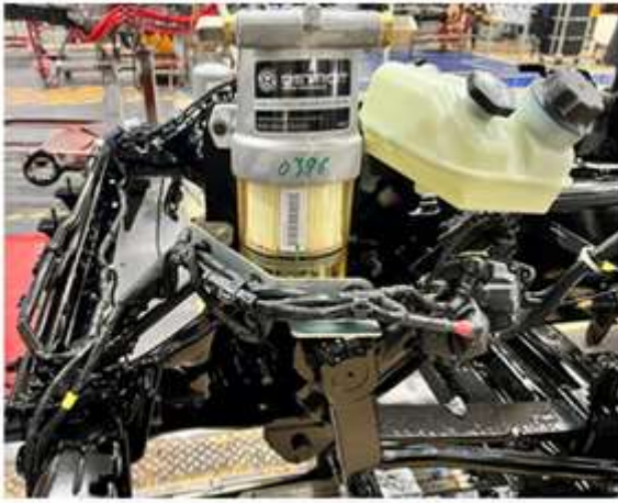
Figure 1. Current Detroit-Racor and FWS- APS Wiring Bracket affecting serviceability.
