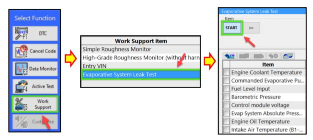
Once the evaporative system leak test is complete, check the DTCs and examine the vacuum value results. Record the value shown in the row labeled MID: \$3C, TID: \$C4, and Scaling ID: \$FE. This value should be lower than -0.26 PSI.
