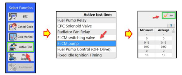
Once the ELCM Pump Active Test has been performed for a period of 35 minutes or more, repeat the Evaporative System Leak Test outlined in STEP 6. Check the DTCs and the vacuum value results.
