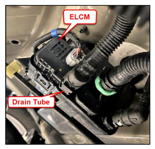
Have signs of water or oil been detected withing the ELCM drain tube?
