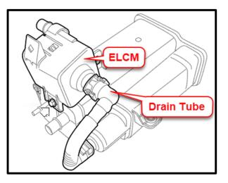
Have signs of water or oil been detected withing the ELCM drain tube?
