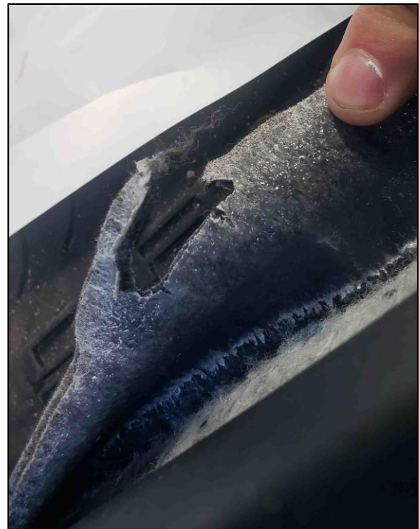
Figure 2. Torn Carpet Loop
