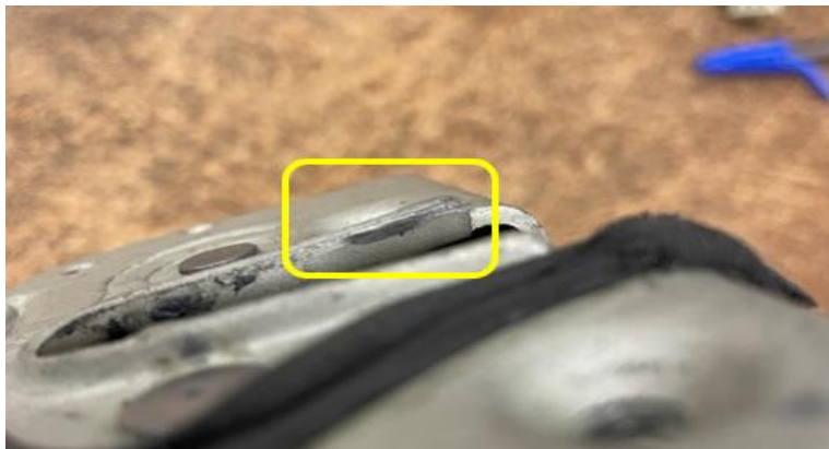
Fig 1. Wear on door latch edge from striker contact.
