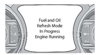
**FUEL AND OIL REFRESH MODE** Since it is possible to operate this vehicle for extended periods without running the gas engine, the fuel within the tank can become stale and/or the engine oil's lubricating properties can be reduced as the vehicle's engine is not operating under its normal engine operating temperatures.
