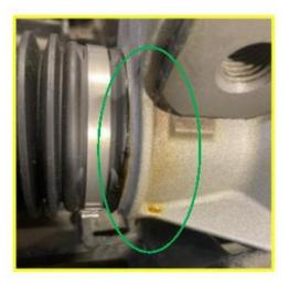
**Discussion**: Minor wetness shown in the above image is normal and part of the manufacturing process of installing he tie rod boots. The wetness near the tie rod boots is normal and would not indicate an EPS repair/replacement is needed. The EPS unit does not contain any oil or grease that can leak out.
