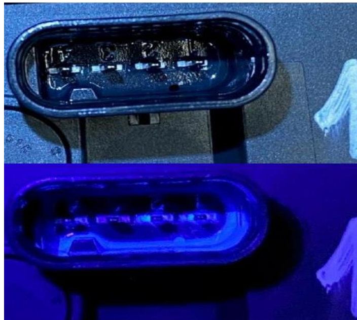
Fig 2. Glow of dielectric grease under a UV black light.
