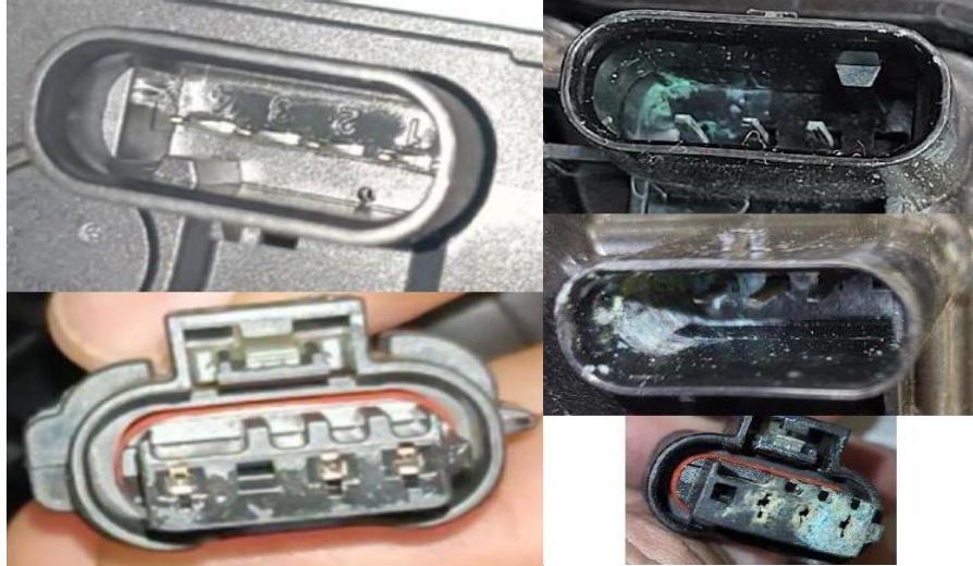
Fig 1. Normal condition left. Corrosion on right.
