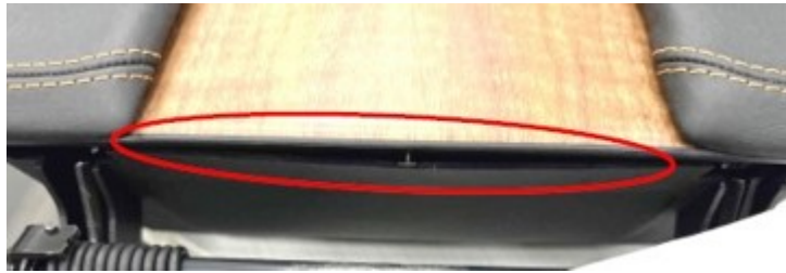
Fig. 1 Console Lower Cover Separating
