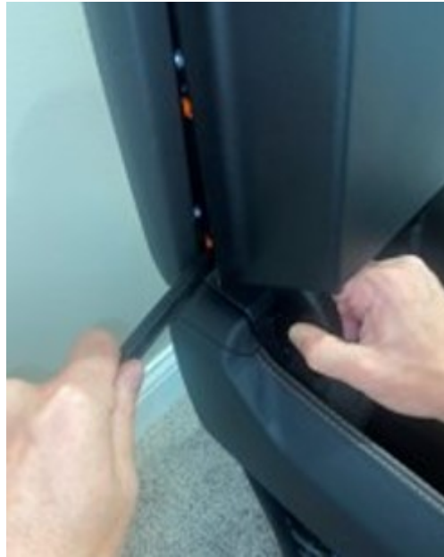
Fig. 2 Lower Cover Removal
