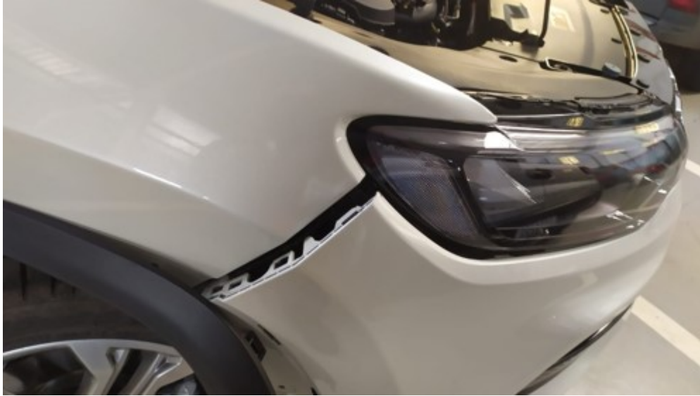
Fig. 2 Front Fascia to be Repaired
