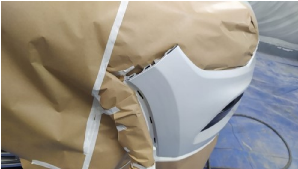
Fig. 5 Taped Off Area to be Painted
