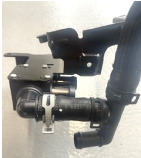
Fig. 2 Incorrect Hose #1 Location
