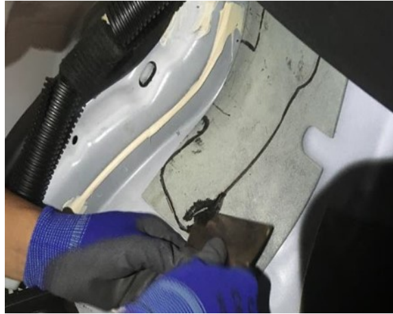
Fig. 3 Deadner Material to be Removed
