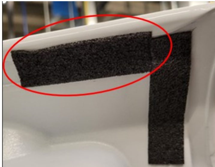
Fig. 2 Foam Pad Installed
