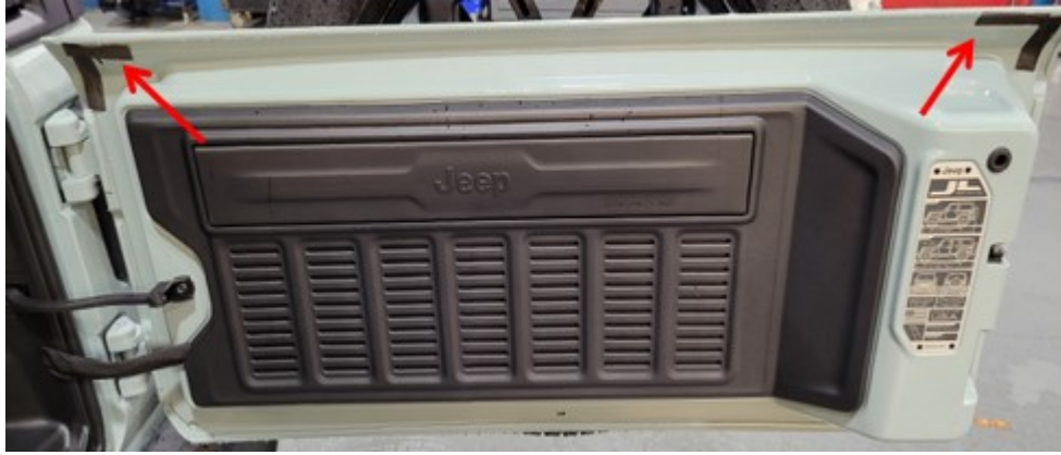
Fig. 3 Foam Pad Installation Complete
