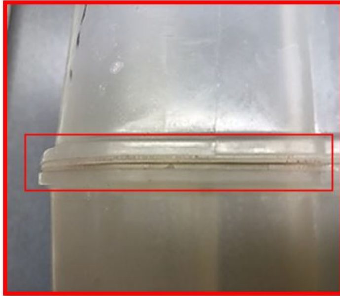
Fig. 1 Coolant Leak Area
