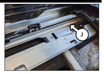
13. Install the new inner curve guide (E) into the grooves and slide inward to set.
