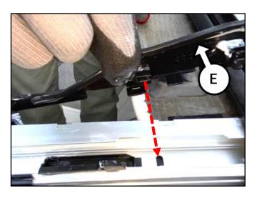
14. Temporarily install the new outer curve guide (F) into the groove and slide outward.
