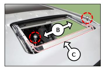
Using a flathead screwdriver, press the lock key
