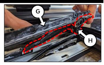
8. Disconnect the driving wedge assembly (H) from the locking side (I), by lifting the wedge assembly and pushing towards the inside of the vehicle, as shown.
