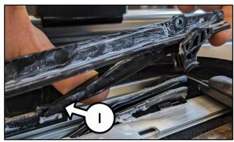
To remove the mechanism sub-assembly (G), push the mechanism sub-assembly towards the front of the vehicle, twisting mechanism sub-assembly at an angle and lifting up.
