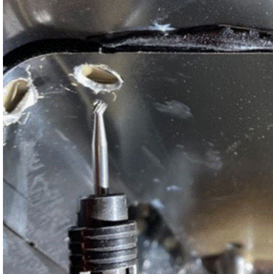
Figure 9. Removing residual primer from inside the drilled area.
