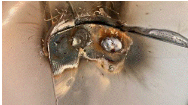
Figure 12. All 3 holes welded completely closed.
