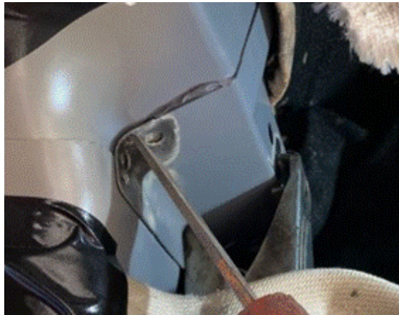
Figure 10. Eliminating any gaps before welding.
