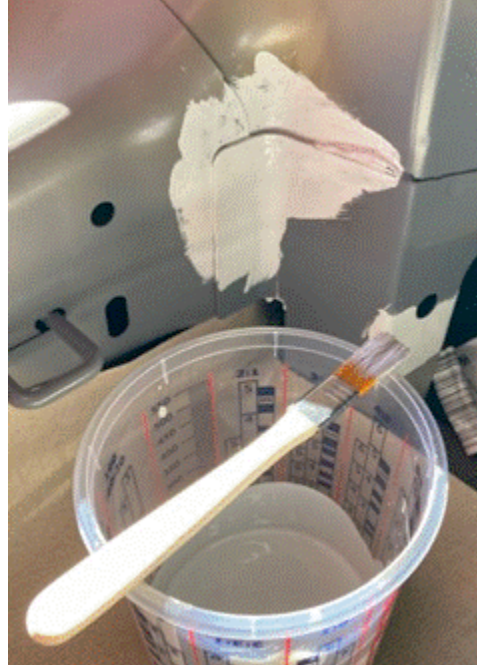
Figure 13. Welded surfaces cleaned and prepped. Corrosion protection restored.
