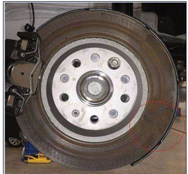
Figure 8: Corrosion, brake pad stuck to brake rotor.
