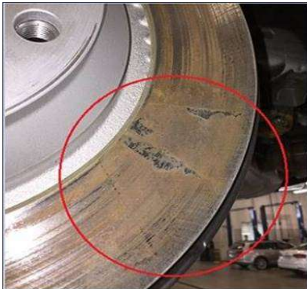
Figure 7: Corrosion, brake pad stuck to brake rotor.
