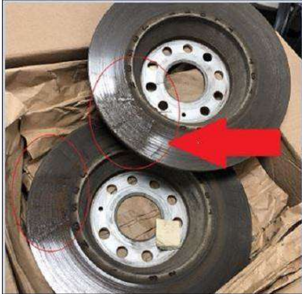
Figure 9: Brake pad stuck to brake rotor
