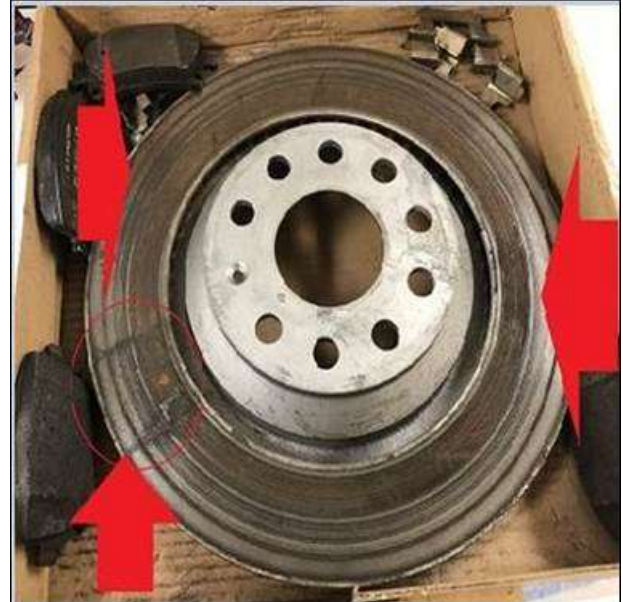
Figure 6: Corrosion, brake pad stuck to brake rotor.
