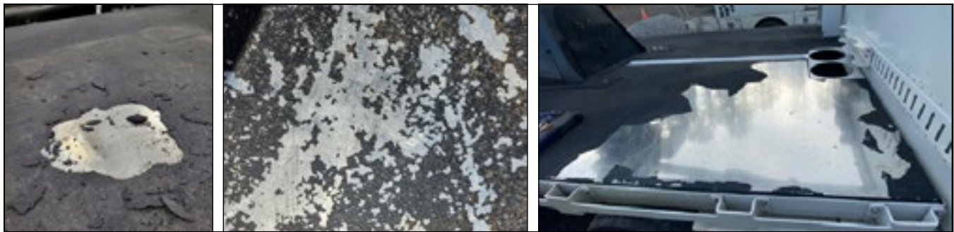
Figure 1 — Examples of Delamination
