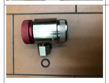
13. Only the R134a adapters fit the quick disconnects of the AC machine.
