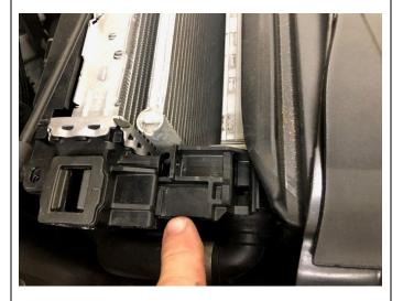
11. There are plastic push tabs that must be depressed to release the AC condenser from the cooling module. This is on the passenger's side.
