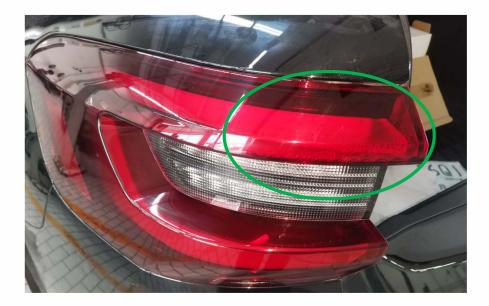
The example shown below is demonstrating a taillight which has excess water entry, beyond normal condensation. Note water across entire lens of the taillight, rather then along the edges alone. This taillight would require correction. This SIB does not apply to taillights which are defective.
