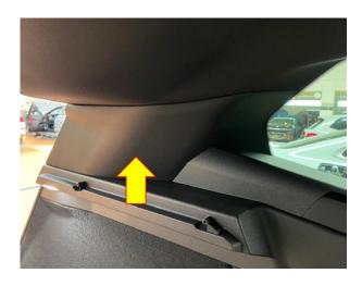
When driving on rough roads, a "cracking" sound can be heard coming from the D-pillar trim panel. The noise can occur on both left and right-side panels.
