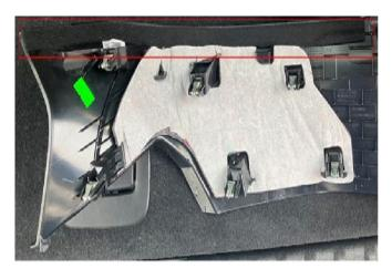
2. Using a thin layer of felt tape, apply it to the top of the D-pillar trim panel as shown in the photo (red bordered area at top).
