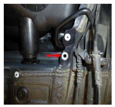
Using a suitable tool (flat countersink), machine the front contact area to bare metal on both the left- and right-hand sides of the body until they are smooth.
