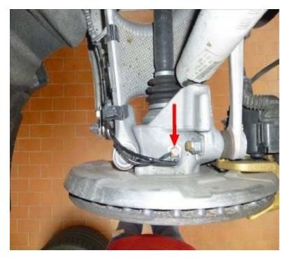
Use the existing mounting bolts to bolt the ground cable (500 mm) from the ESD ground cable set onto the relevant rear wheel speed sensor (L and R). Torque to 8 Nm.
