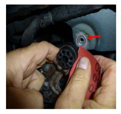
To improve conductivity, clean the contact area for the DSC bracket with sandpaper.
