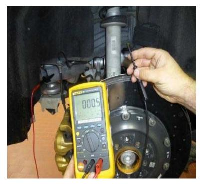
Use an ohmmeter to check that all of the newly attached ground cables are working (zero resistance between the wheel hub and the vehicle's ground).
