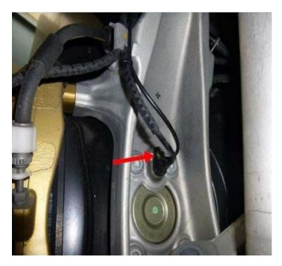
Use the existing mounting bolts to screw the ground cable (750 mm) from the ESD ground cable set onto the relevant front wheel speed sensor (L and R). Torque to 8 Nm.
