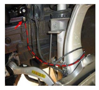
Route the ground cable along the wheel-speed sensor cable. Use a hex bolt (M6x14, 9 905 525) and a hex nut (M6, 9 915 702) to screw the other relevant ground cable end onto the prepared body attachment point (8 Nm). Secure it using the cable straps (1 372 391).
