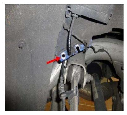
Using a suitable tool (flat countersink), machine the rear contact area to bare metal on both the left- and right-hand sides of the body until they are smooth.
