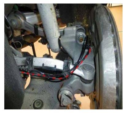
Route the ground cable along the wheel-speed sensor cable. Use a hex bolt (M6x14, 9 905 525) and a hex nut (M6, 9 915 702) to screw the other relevant ground cable end onto the prepared body attachment point (torque 8 Nm). Secure it using the cable straps (1 372 391).
