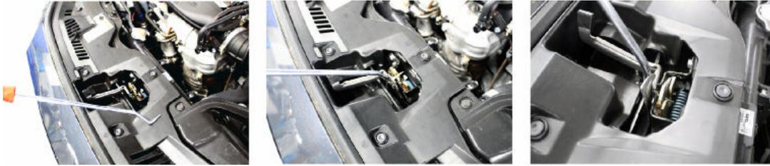
3. Open the front doors, and then manually engage the latches.
