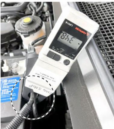
7. Test parasitic draw with the ignition OFF.
