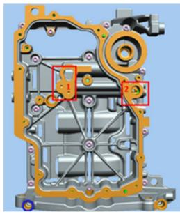
Caution: If oil pump replacement is needed, ensure the three oil pump oil holes (Area 1) and OCV mounting hole (Area 2) are free of debris BEFORE installing the oil pump and OCV. If debris is found, remove with a lint-free cloth or brush that will not scratch the surface.
