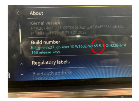
If the build number is less than Y167, update the radio software.
