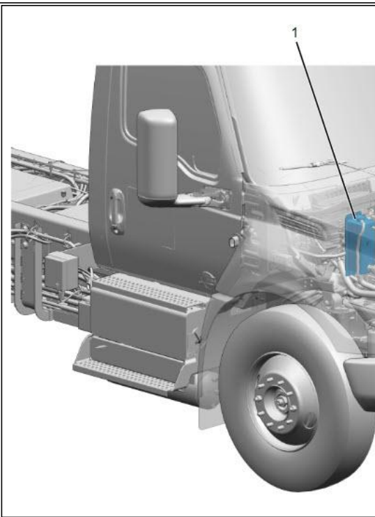
Figure 2: eMV Surge Tank Locations
