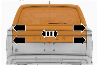
Target gap: Equal values (the component should be centered).
