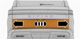
Target gap: Equal values (the component should be centered).
