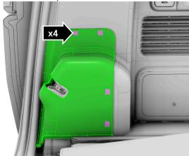
c. On both sides: Loosen the highlighted fasteners to adjust the component.
