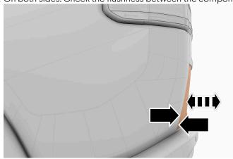
Target flushness: Lower liftgate 0.5-3.5 mm underflush to the bodyside.
