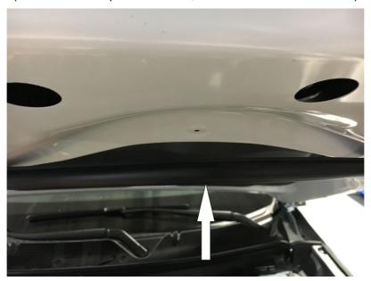
To correct this concern, reattach the weatherstrip or replace it with a new one if it is damaged.
