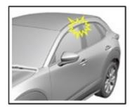
To eliminate this concern, the fixing force and durability of the glass run channel against thermal expansion and vibration has been improved. The shapes of the front and rear glass run channels and the rear garnish lip have been changed to prevent interference.
