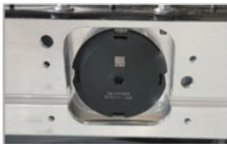
Image 4 – Vent Cap not covered & missing screws
