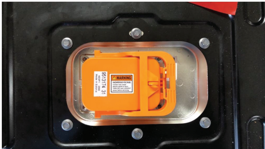
Image 1 – MSD covered properly, showing the preferred method through utilization of P/N 9513174 to secure the MSD housing. (Code 502)
