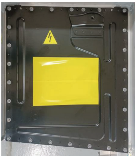
Image 2 – MSD covered properly, another acceptable method with colored tape. Note that the entirety of the MSD opening should be covered to avoid entry of debris. (Code 502)
