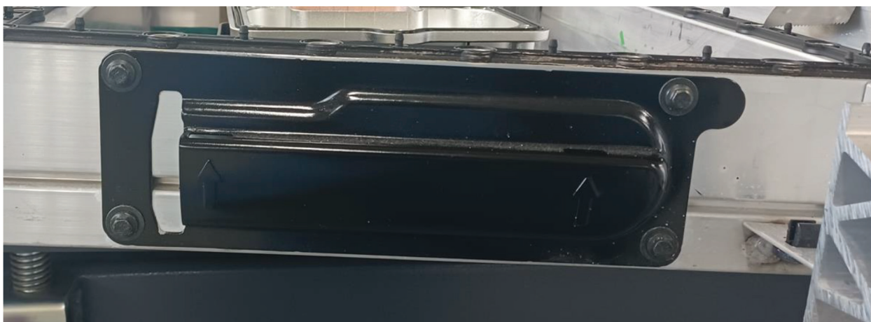
Image 5 – Proper Vent Capping for new BEV pack variant (after chassis number 66548 for 534) with P/N 32299402
