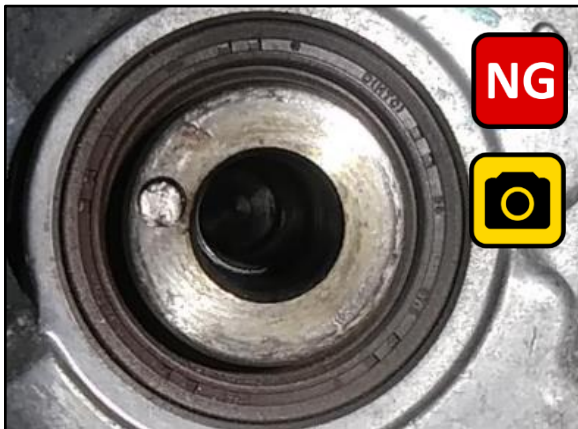
Damaged crankshaft end.
