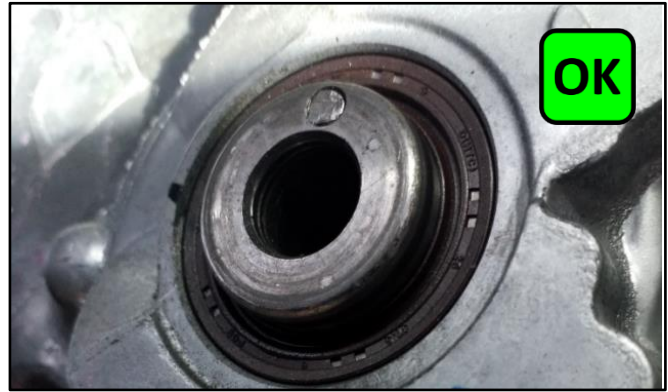
No damage to crankshaft end.
